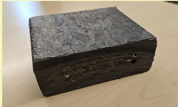
Span and load guidance based on laboratory flexural testing of LL Plastic recycled plastic joists (50 x 120 mm) using a 1000 mm support span and conservative safety factors.
